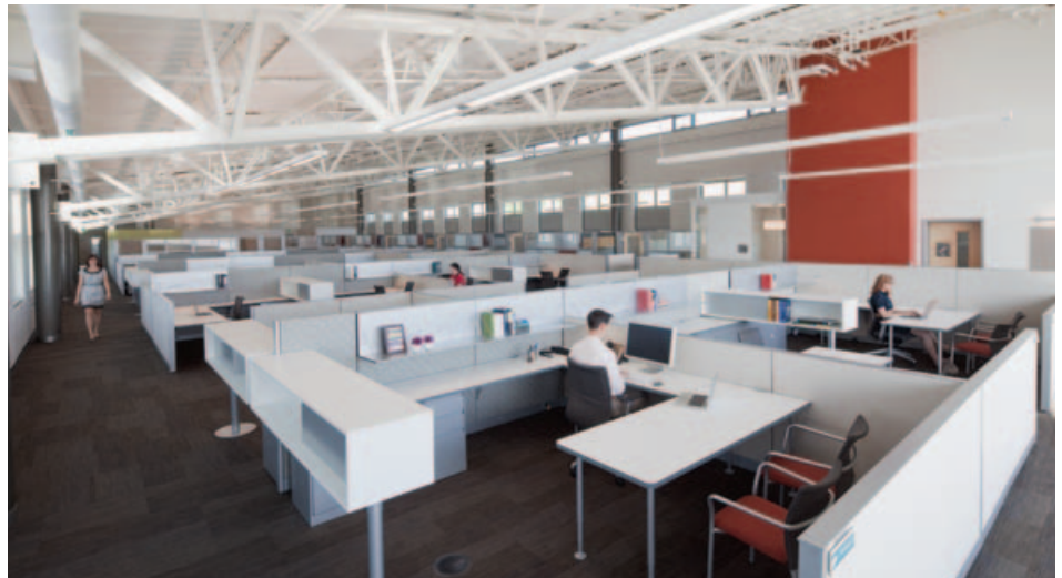
The low profile of modular workstations allows for maximum daylighting. (Courtesy of Frank Ooms, Frank Ooms Photography)
